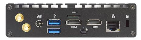
The JETWAY HBJC420P891 Series adopts the Intel® Gemini Lake SoC processor. The board has one 260-pin DDR4 2400MHz SODIMM up to 8GB memory. JNP891 Series equipped with DDR4 SODIMM slot and M.2 (M-key, 2242) which is suitable for most of the Digital Signage applications.
